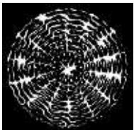
The 18th century German physicist and musician Ernst Chladni first demonstrated a way to make sound vibrations visible. When he drew a violin bow around the edge of a plate covered with sand, the sand formed intricate geometric patterns which today are termed “Chladni figures.” (Examples of Chladni figures are found above and below.)
